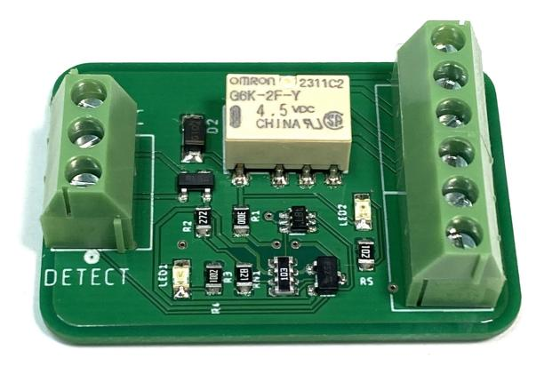
This is the \*\* NEW \*\* DPDT (Double Pole, Double Throw) relay from Model Train Technology that works with our Precision Detector eco-system. You power the coil side (left side) with 12VDC and connect the single yellow signal wire to the DETECT from the output from the Precision Sensor. The right side are the 6 connection to the contacts of the relay. There is a blue LED that tells you the board is powered. When the coil is activated, a green LED lights.
