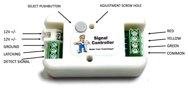
When you plug in power the blue internal LED will light. The green LED or FIBER output will light.
