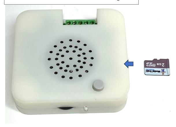
The socket for the TF card is spring loaded. Slide in to insert. To remove, push in slightly and let the spring push the card out.
