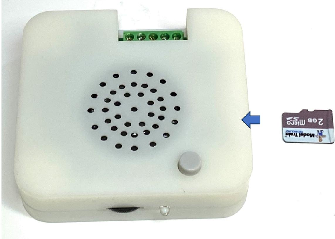
The socket for the TF card is spring loaded. Slide in to insert. To remove, push in slightly and let the spring push the card out.
